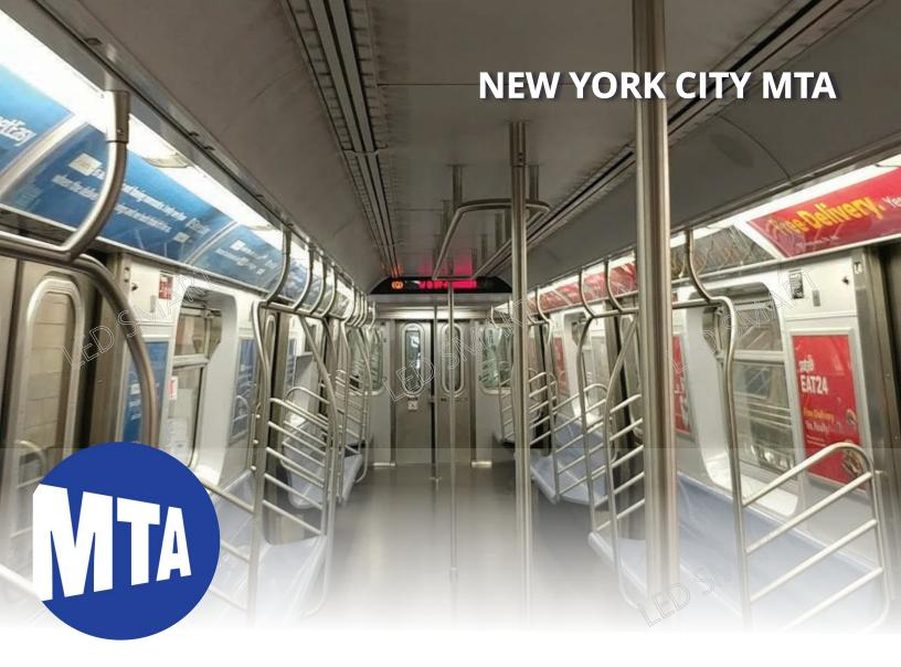
The New York City Transit department uses LED Smart, custom LED lighting system to retrofit their Alstom, Bombardier and Kawasaki R142, R142A, and R160 cars. MTA NYCT is in the process of retrofitting these 3,138 cars with the best in LED technology, the LED Smart RLR Series.
